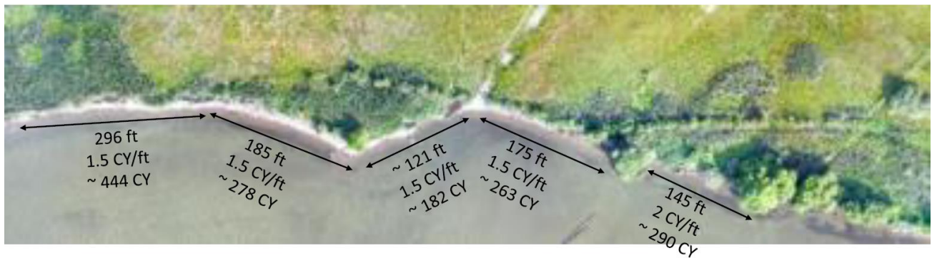
Figure 1 illustrates the linear beach segments of the existing dynamic equilibrium beach and volume of 3" minus screened pit run (small rocks) needed to reinforce the beach.
