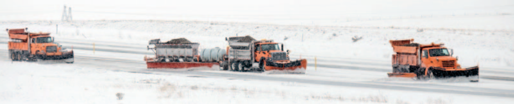
When snow starts covering Montana highways, MDT crews head out in snowplows, including “double-winged juice trucks” (fitted with a pair of 11-foot plows and carrying tanks of salt-sand-magnesium chloride solution to spray on roads).
