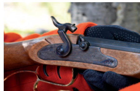
A traditional percussion cap version with its external, indirect ignition system.
