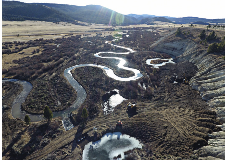
RESTORED TRIBUTARY Above: On French Creek, a Big Hole River tributary, crews reconfigured 4,000 feet of stream channel away from an eroding hillside. They created new wetlands to store water and planted willows and other streamside vegetation that shades the water while providing browse for moose, elk, and other wildlife. Below: Landing a big rainbow near Wise River.
