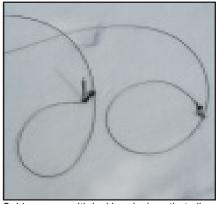
Cable snares with locking devices that allow the snare loop to close one way and tighten around an animals neck.
