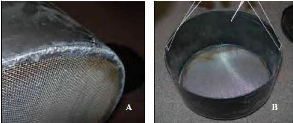
Figure 16. A) Mesh melted into the plastic bucket. B) Finished egg basket
