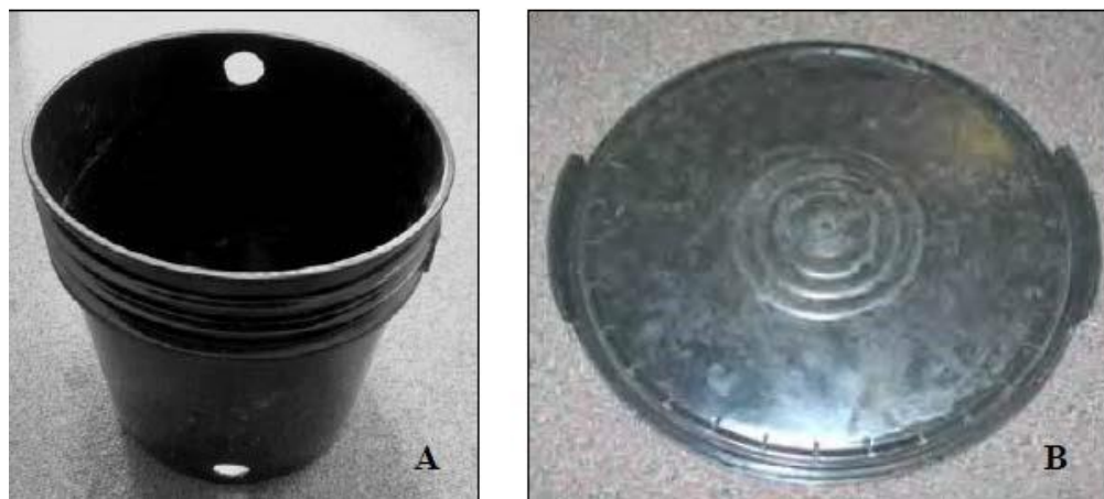
Figure 15. A) Bucket with hole drilled into opposite sides. B) Bucket lid with all but 2 tabs removed to provide easy access to inner workings.
