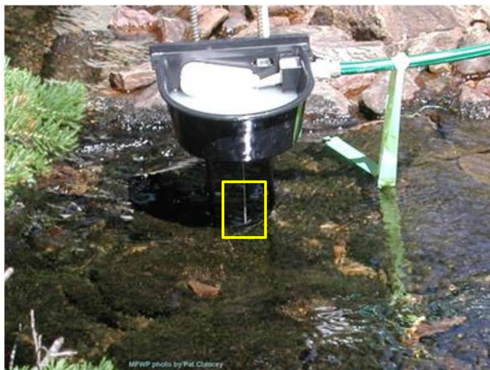
Figure 2-6. Close-up of the Montana bucket system trickling CFT Legumine/stream water solution into a stream. The stream of CFT Legumine and stream water solution is visible in the yellow box.
