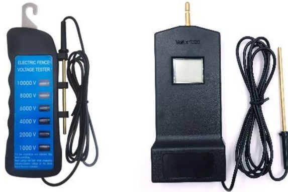
Figure 9. Two common styles of electric fencing voltage meters, LED (left) and digital (right).
