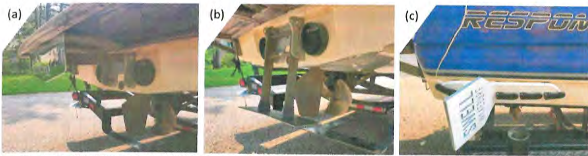
Figure 6. Malibu Response LX hydrofoil in the (a) stow position and (b) deployed down position. (c) Installed aftermarket wake shaper (Swell Wakesurf- Wakesurf Creator 2.0).
