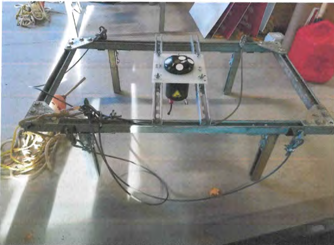
Figure 5. An ADCP secured to the custom-built pad and ready for deployment. The four lifting cables and lift rope can also be seen in the image.
