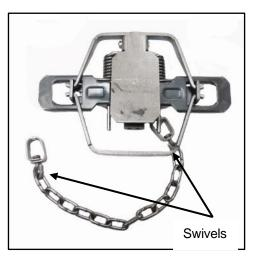
While many Montana trappers already incorporate these swivels, adding an attachment point (if one is not present) and swivel on a trap's base plate could cost between \$ 0.35 and \$1.50 per trap and take 10 minutes to install.
