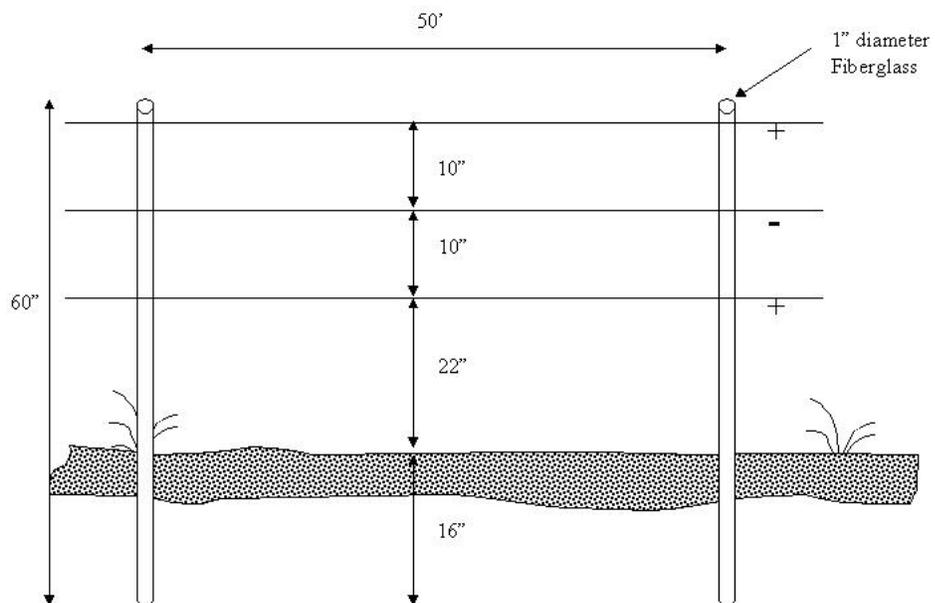
**Figure 2.** Electric fence design detail cont.
