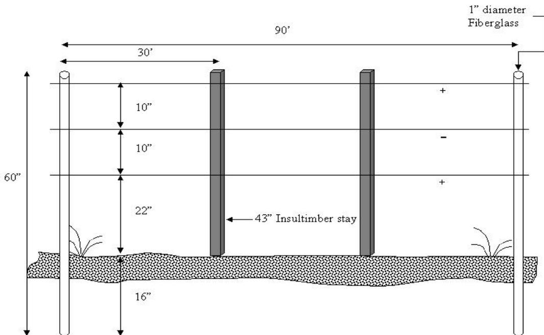
**Figure 2.** Electric fence design detail cont.
