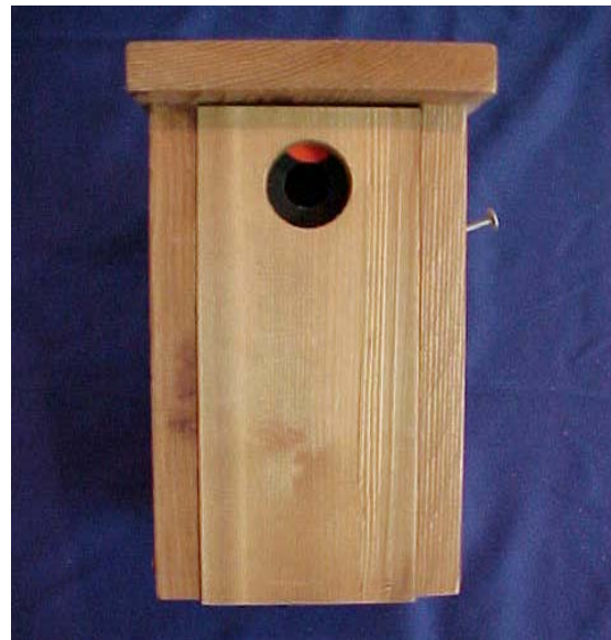
Figure 10 A Van Ert-style starling box trap. The red dot appears in the window when the trap is sprung.
