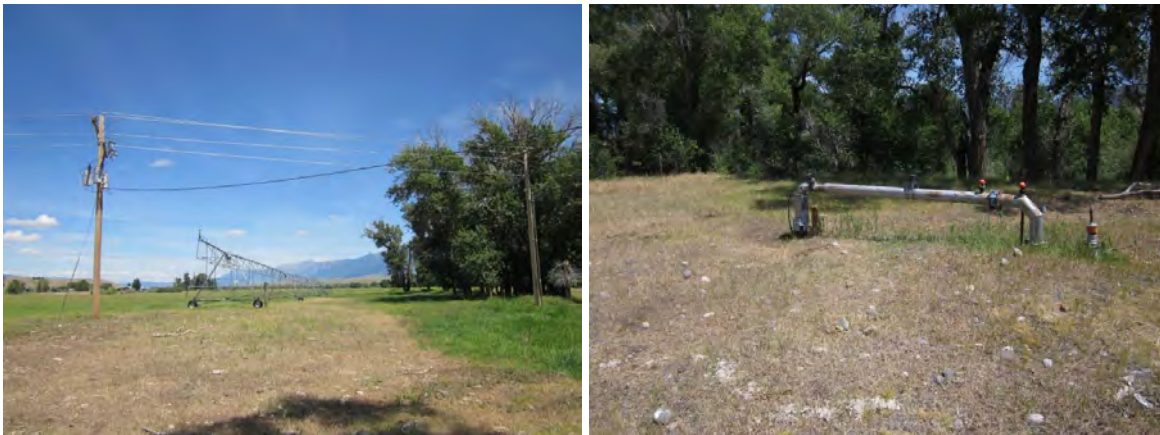
FIGURE 64. CENTER PIVOT INSTALLED AS A WATER SAVINGS MEASURE FOR NORTH FORK FRIDLEY CREEK (L) AND PUMPING STATION SUPPLYING WATER TO CENTER PIVOTS (R).
