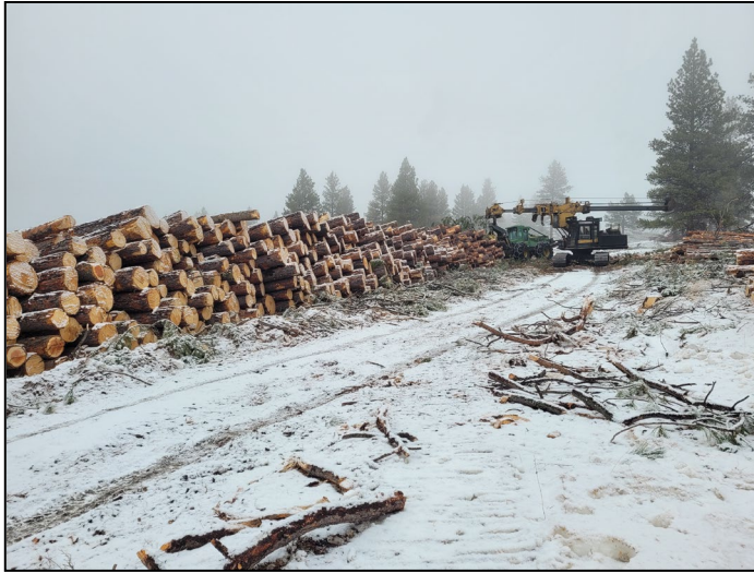
Figure 9 – Stroke-boom delimeter processing encroachment trees from grass/shrublands to improve winter range. January 2022. Image: J. Parke
