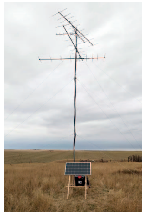
PING, PING, PING Key to the Motus Wildlife Tracking System are a series of stations fitted with antennae that pick up the unique signal of each tagged bird that flies past.
