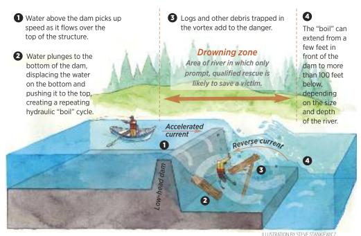
TRAPPED Low-head dams don't appear dangerous. Because the structure is hidden underwater, boaters, kayakers, and other floaters can't judge how deep the water is above and below the damor how fast it moves over the top. Also hidden is the deadly hydraulic, caused by the large volume of water flowing over the structure. Victims are usually trapped between the two current forces.
