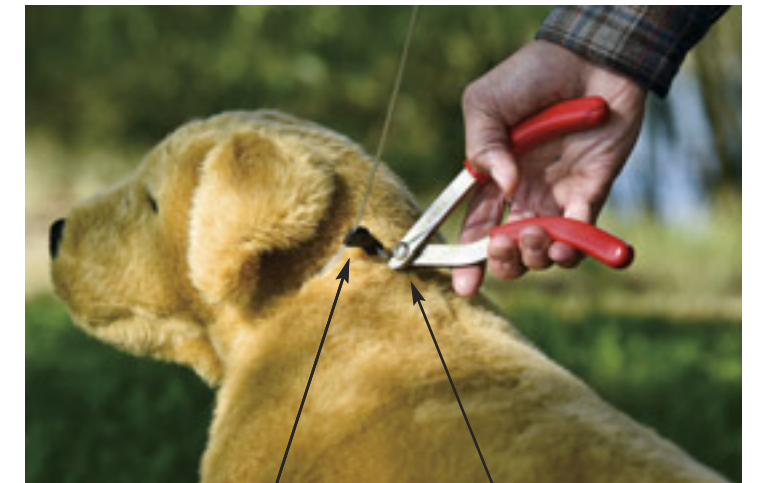
Toggle the locking mechanism to loosen the cable.
