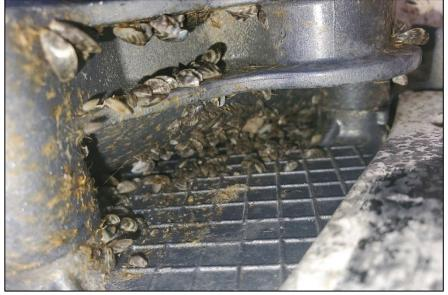
PHOTO 3. MUSSELS ON WATERCRAFT INTERCEPTED AT WIBAUX INSPECTION STATION
