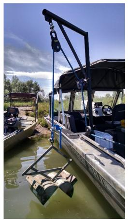
Figure 7: Ponar dredge used to sample sediment in Tiber Reservoir
