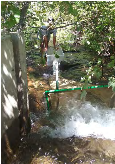
FIGURE 79. EXAMPLE OF A FRY TRAP.
