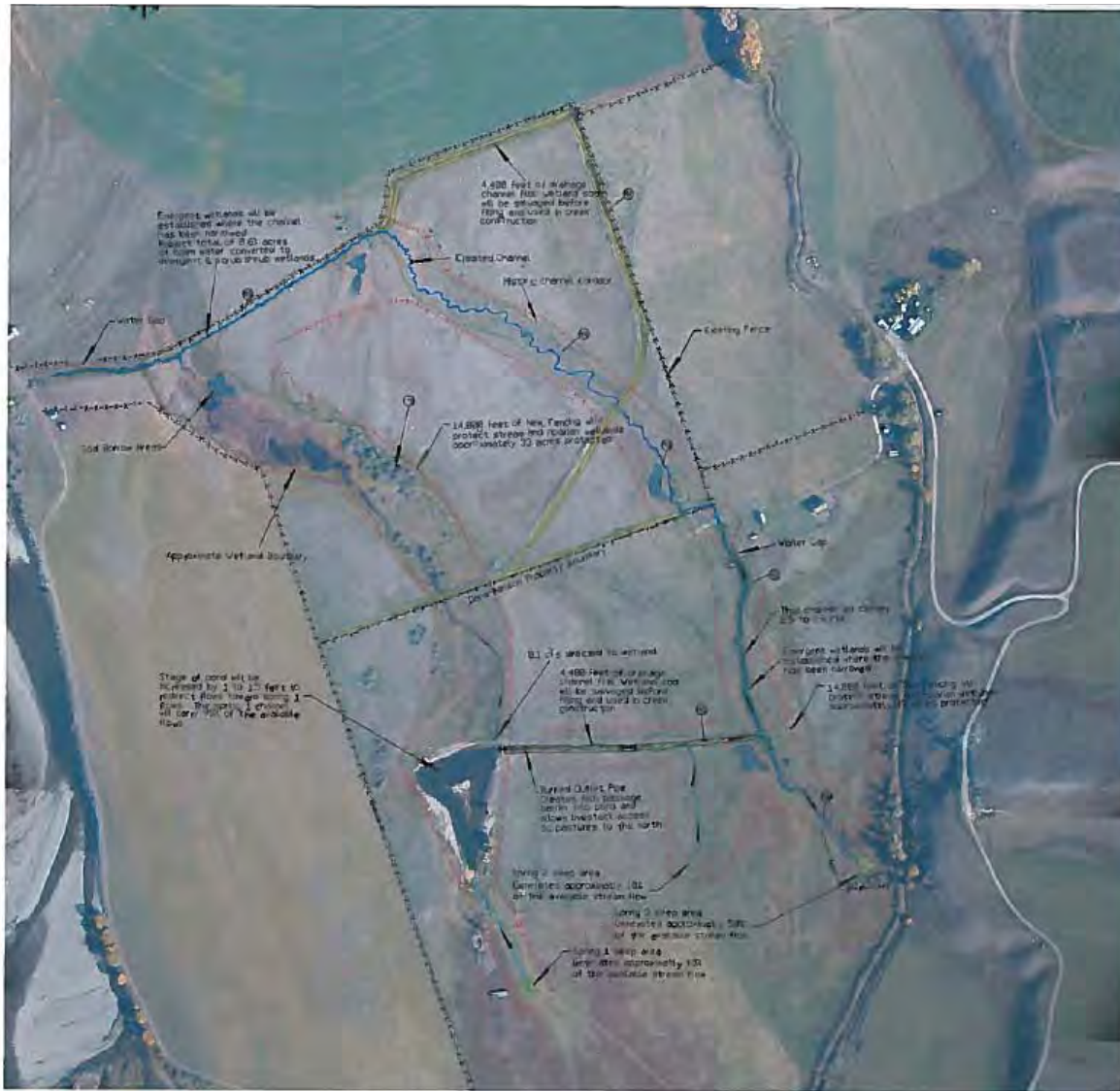
FIGURE 65. DESIGNS FOR THE NELSON/DANA SPRING CREEK RESTORATION.
